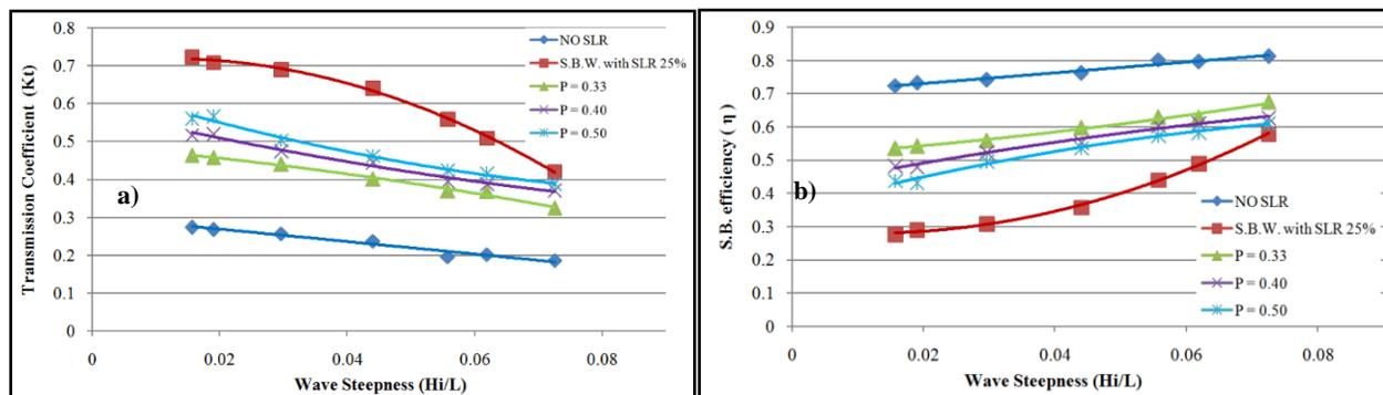
Figure 6. a) Single wave screen influence on the transmission coefficient ( $K_t$ ), b) Single wave screen influence on S.B.W. efficiency ( $\eta$ ).
