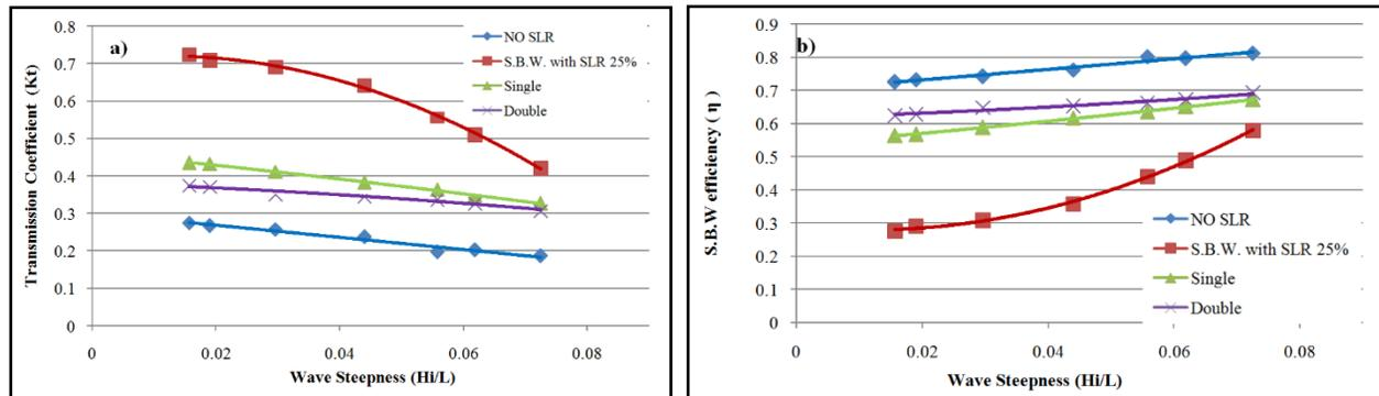
**Figure 11. a) The influence of single and double wave screens on the transmission coefficient ( $K_t$ ), b) The influence of single and double wave screens on S.B.W. efficiency ( $\eta$ ).**
