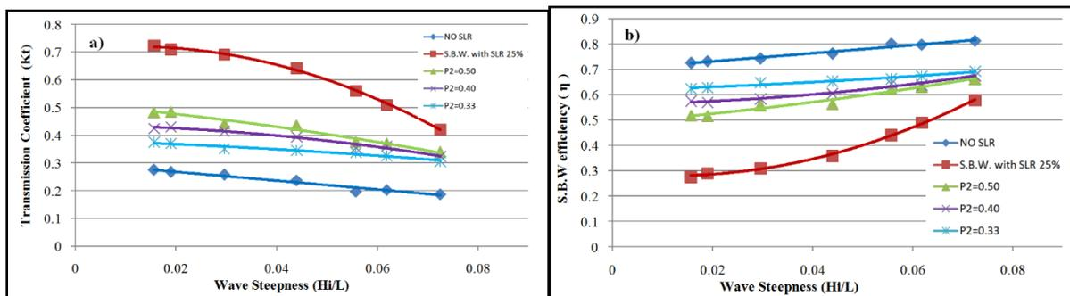
Figure 10. a) The porosity influence of leeward screen on the transmission coefficient ( $K_t$ ), b) The porosity influence of leeward screen on S.B.W. efficiency ( $\eta$ ).
