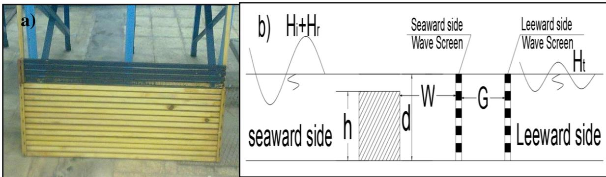
Figure 4: a) Horizontal slats wave screen model, b) The used wave screens in the leeward side of the S.B.W. model.
