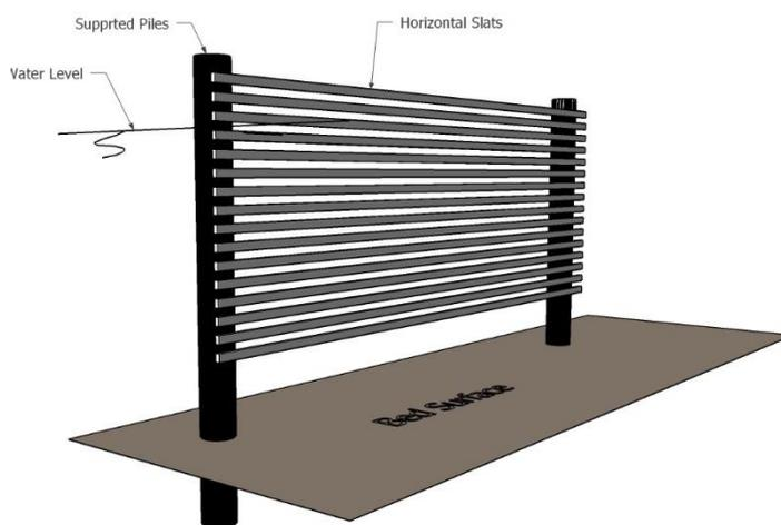
Figure 1. Schematic diagram of a horizontal slats wave screen
