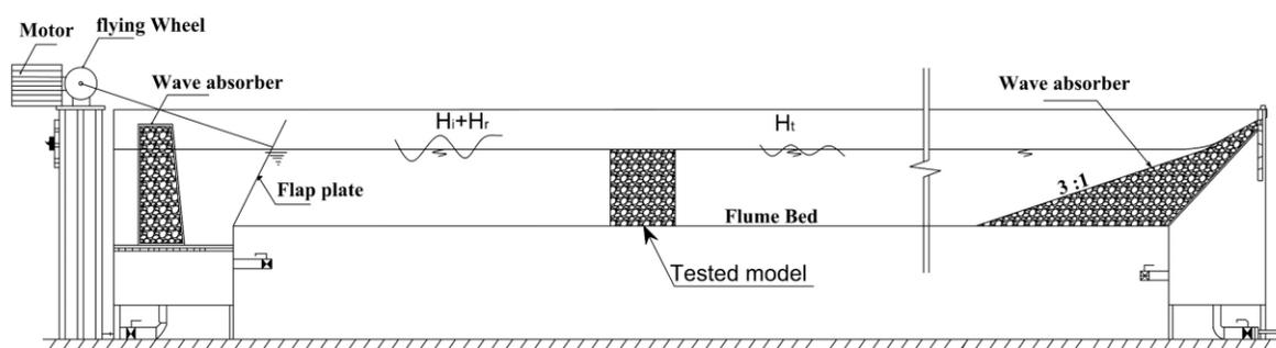
Figure 2. Schematic diagram of the wave flume
