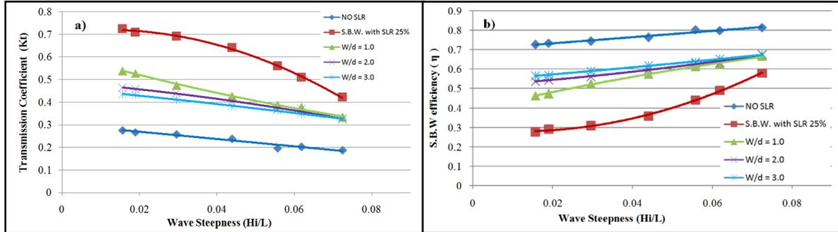
Figure 7. a) The influence of relative distance of screen on the transmission coefficient ( $K_t$ ), b) The influence of relative distance of screen on S.B.W. efficiency ( $\eta$ ).
