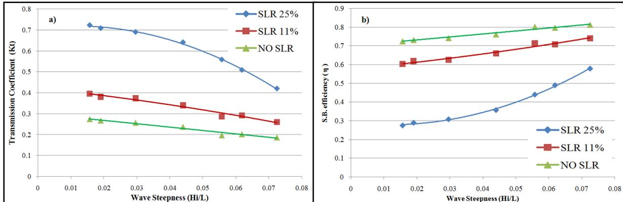
Figure 5. a) SLR impact on the transmission coefficient ( $K_t$ ), b) SLR impact on S.B.W. efficiency ( $\eta$ ).
