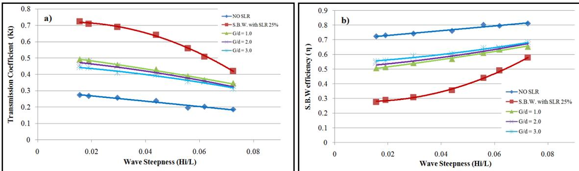
Figure 9. a) The influence of the relative gap of double wave screens on the transmission coefficient ( $K_t$ ), b) The influence of the relative gap of double wave screens on S.B.W. efficiency ( $\eta$ ).
