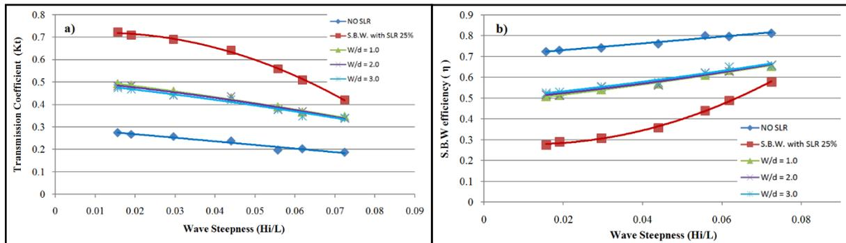
Figure 8. a) The influence of relative distance of double wave screens on Transmission coefficient ( $K_t$ ), b) The influence of relative distance of double wave screens on S.B.W. efficiency ( $\eta$ ).
