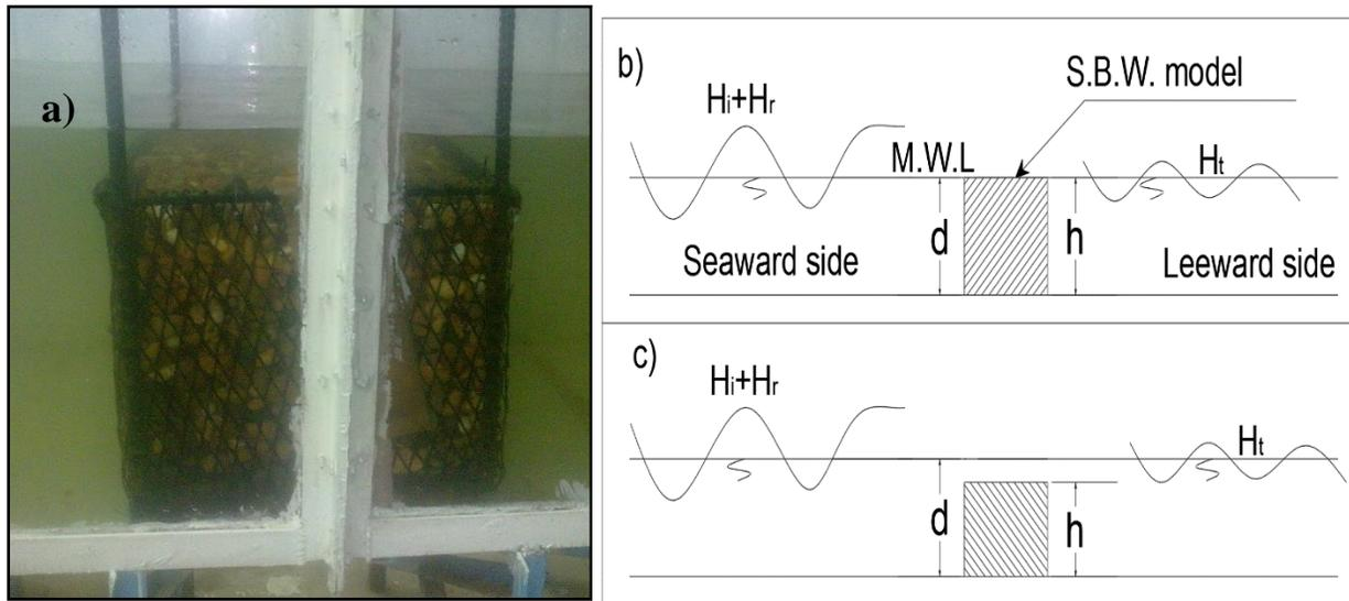
Figure 3, a) The S.B.W. model, b) The original case with no impact of SLR, c) The tested model in case of SLR.
