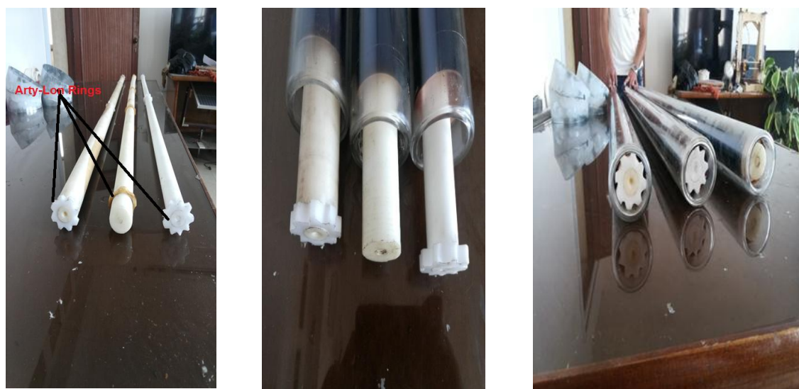
Figure 5. pictures of ERTALON columns inside the ETCs.
