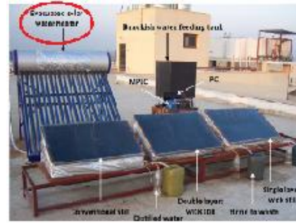
Solar Still and evacuated solar water heater (Omara, Eltawil, and ElNashar 2013)
